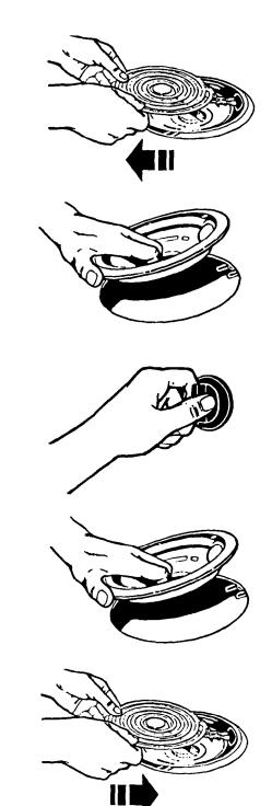
4. When the terminal is pushed into the receptacle as far as it will go, push down the edge of the surface unit opposite the receptacle. The element hold-down clip will keep the surface unit from moving around.
